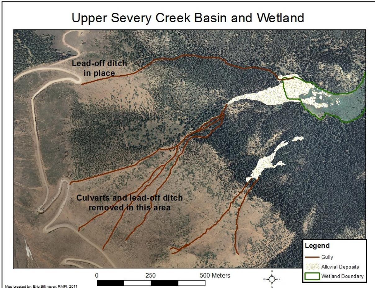
Figure 9. Map showing areas where highway improvements have been made in the upper Severy Creek Basin (base image is from 2005 before paving was completed).
