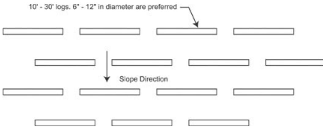
Figure 38. Erosion Log Barriers. (NRCS, 2004).
